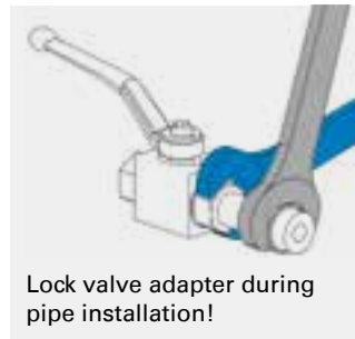
No welding, boring or other modification at the valve!
