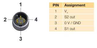
**SCLTSD-xxx-10-07** for temperature and level 1 switching output, 1 analogue output, M12x1; 4-pole
