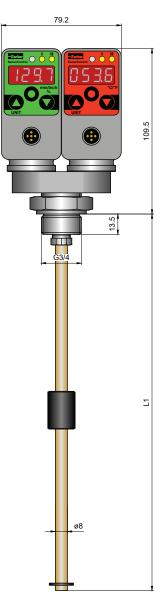
L1 = length of the sensor (mm)L2 = active range (mm)
