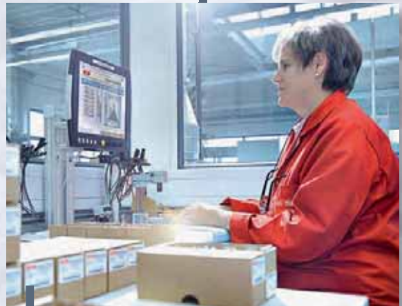
Fully automated switching point adjustment with computer-aided documentation of readings.
