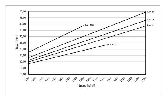
If PAH 63/70/80 run 1800 - 2400 rpm the following conditions apply: Inlet pressure 2 - 4 barg, outlet pressure max. 140 barg for a maximum of 500 hours in between service inspection.
