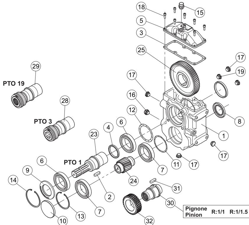
When ordering spare parts, specify reference number, gearbox model, PTO type and transmission ratio.
