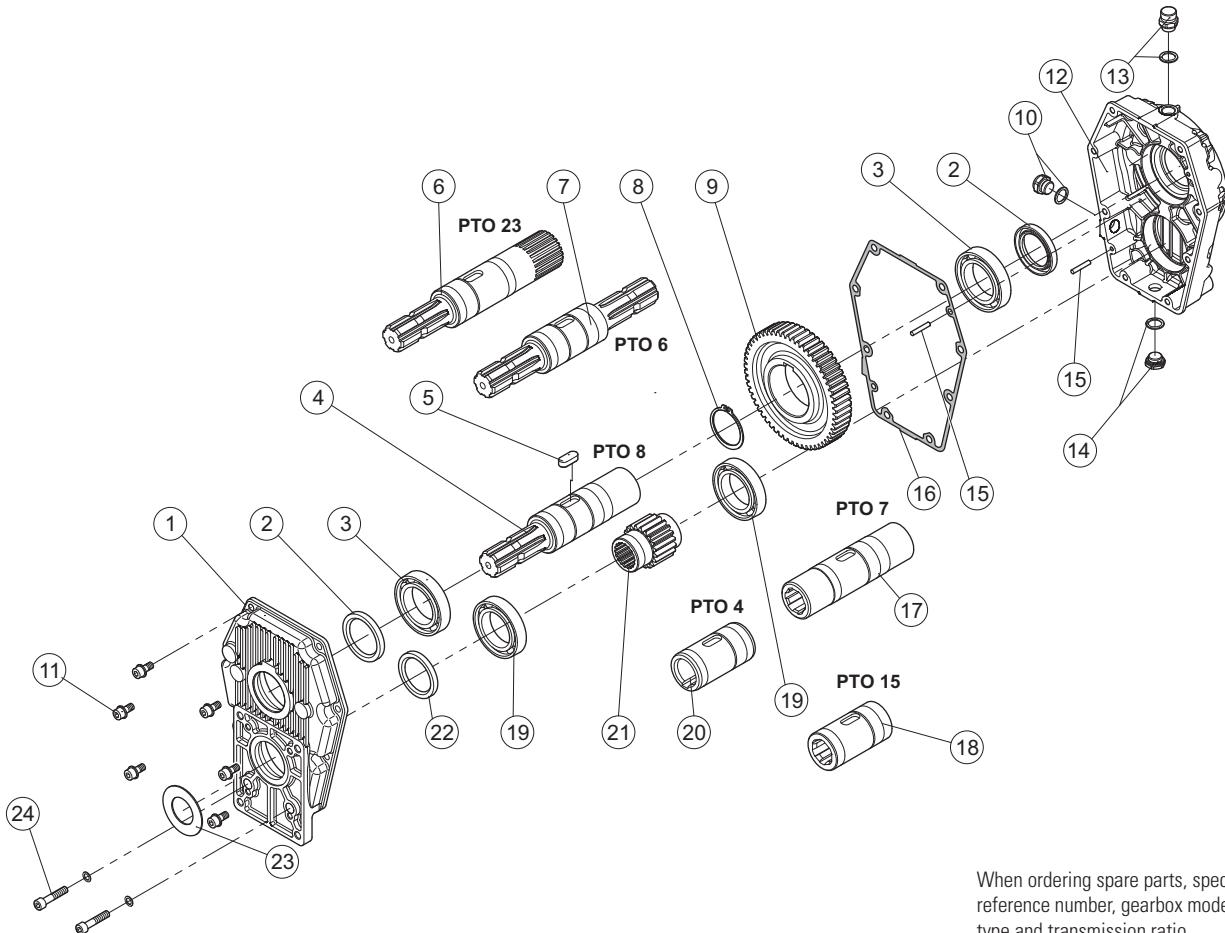
When ordering spare parts, specify reference number, gearbox model, PTO type and transmission ratio.
