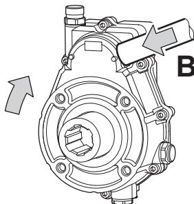
If it is not possible, gearboxes should be bound with a torque arm "B" (see figure). To avoid abnormal stress to the system, the torque arm "B" must be placed as close as possible to the mounting plane (PTO side) of gearbox.
