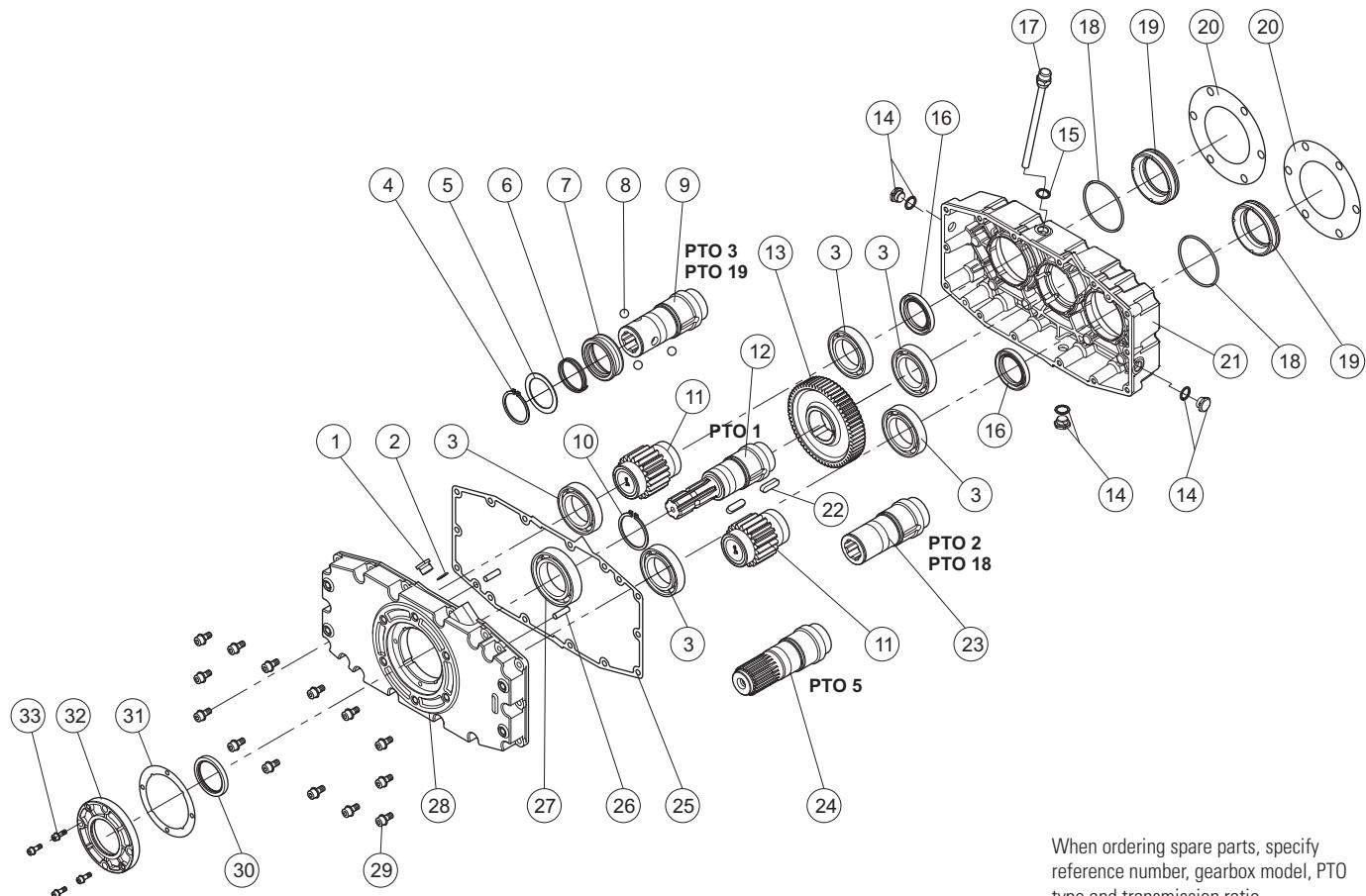
When ordering spare parts, specify reference number, gearbox model, PTO type and transmission ratio.
