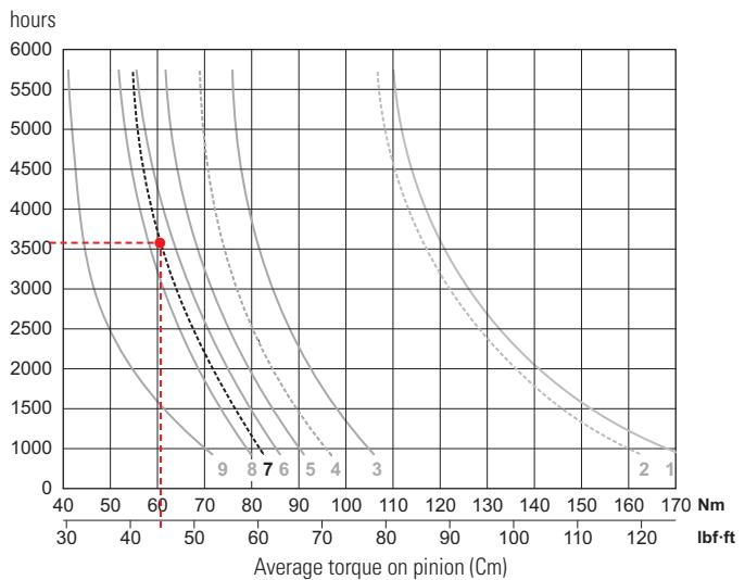
In diagram curve number **7** has to be considered (gear ratio **1: 2.5** at **1000 rpm**). The estimated duration of the average torque of **60.4 Nm** is approximately **3600 hours**.
